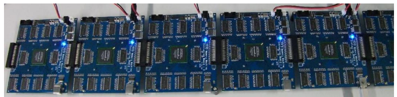
Figure 5 Parallel computing system of FDTD dedicated computers
